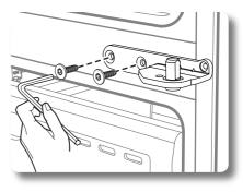
2. After removing one screw and two hex bolts, remove the Middle Hinges. (Unscrew the two hex bolts with the 4.75mm hex wrench.)
